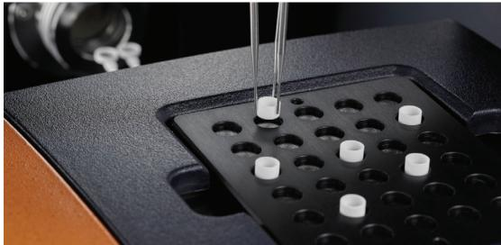
The NEW Discovery SDT features our 30-position autosampler to optimize productivity. Based on our proven Discovery DSC design these rugged autosamplers are cycled extensively in our factory to ensure worry-free operation.
