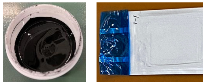
Figure 1. LFP cathode slurry and laminated pouch-type full cell
