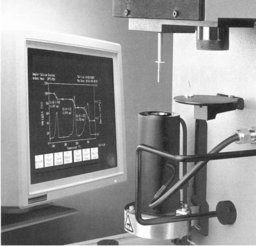
Thermogravimetric analysis (TGA) measurements are used primarily to determine the composition of materials and to predict their thermal stability at temperatures to 1000°C.
