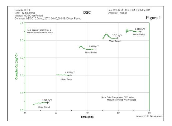
Figure 1 shows the effect of modulation period on a sample of high-density polyethylene. As seen in the data, the measured heat capacity for the 30- and 40-second periods is low by 15 - 20% as compared to the 100-second modulation period. This is due to the mentioned thermal resistances as well as the use of sensor temperature instead of sample or pan temperature in the calculation.
