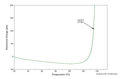
A typical DTUL curve shows a negative dimension change, which indicates upward motion of the fulcrum due to the thermal expansion of the sample. As the temperature rises, there is a downward movement that overcomes the thermal expansion and the sample starts to deform under the load. When the dimension change reads a *positive* 113  $\mu$ m dimension change, that is the temperature we are looking for when reporting DTUL. For the polycarbonate used in this example, the DTUL is about 140 °C.
