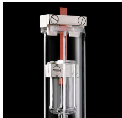
Figure 3. Film/fiber probe for the TMA 450 RH loaded with a film.
