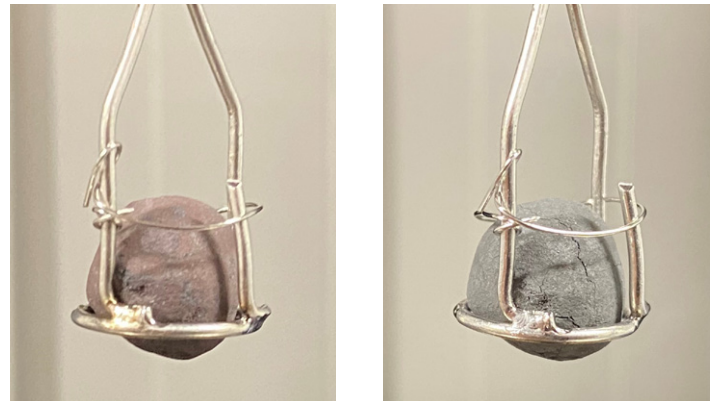
Figure 5. Pellet sample before and after reduction at 1 bar 700 °C
