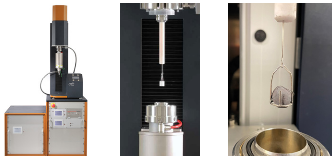
Figure 2. For best performance, the DynTHERM Ceramic Crucible was replaced with a platinum wire holder for the sample pellet
