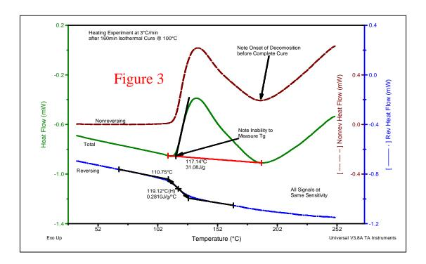
Note that it is not possible to see or measure the glass transition of the partially cured epoxy in the Total signal, which is equivalent to what would be obtained by standard DSC. The reason for this is that the endothermic glass transition is hidden by the more energetic exothermic reaction.
