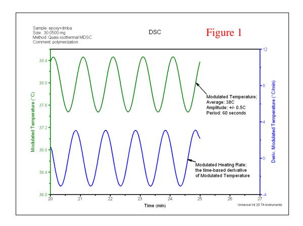
Even though the average temperature remains constant in MDSC, it is possible to measure heat capacity because of the modulated heating rate.
