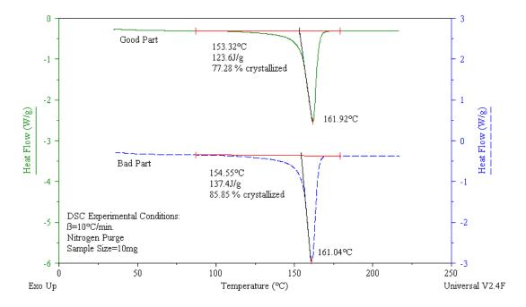
**D**SC measures the temperatures and heat flows associated with transitions in materials as a function of temperature or time in a controlled atmosphere. This technique provides quantitative and qualitative information about physical and chemical changes that involve endothermic or exothermic processes, or changes in heat capacity.
