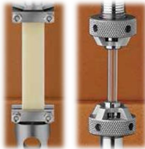
Rectangular and cylindrical torsion
